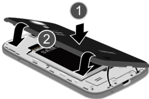
2. Press down along the edge of the back cover (3) until you have a secure seal.
