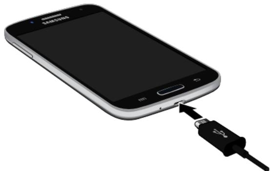
1. Plug the flat end of the Travel Charger into the charging/USB port and the other end into a standard AC wall outlet.
