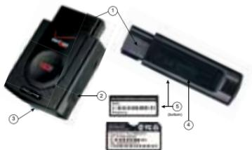
1. OBD connector (plugs into vehicle's OBD-II port)
