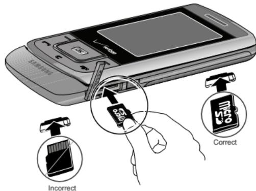
2. Push the microSD card into the slot until it locks into place.
