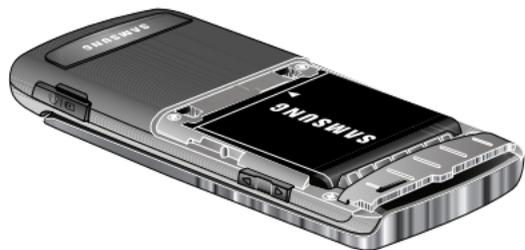
3. Slide the battery cover up until it snaps into place.
