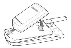
Gently push the top end of the battery down (The top end of the battery displays the word Samsung in raised letters.) until you hear it click into place.
