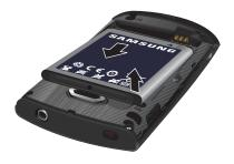
3. Lift the battery up and out of the phone.
